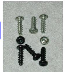
**Tin-Zinc**— Tin-zinc is the newest of the alloys. It offers excellent corrosion protection. It is often used as a replacement for cadmium due to its excellent conductivity and lubricity. It offers excellent solderability and superior ductility. It is rapidly gaining in popularity particularly in the automotive industry and is very often used in grounding applications. It is a non-cosmetic finish.
