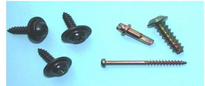
**Zinc-Iron**— Zinc-iron offers good weldability and ductility making it a good choice for components that will undergo subsequent manufacturing operations. It is often used on parts that are to be painted. It is the least expensive. Zinc-iron clear offers a good cosmetic appearance. Zinc-iron is most suitable for black chromate.
